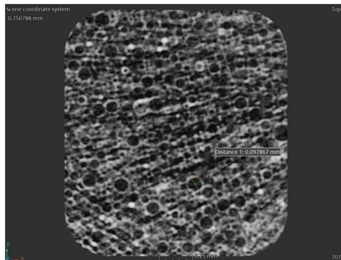
**Figure. 4.** Internal structure of spherulite in the upper plane with measurement of one pore
