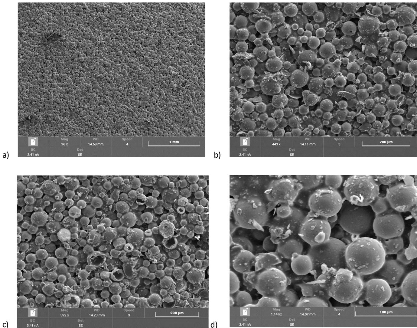
Figure. 6. Surface of the nano-insulation coating
