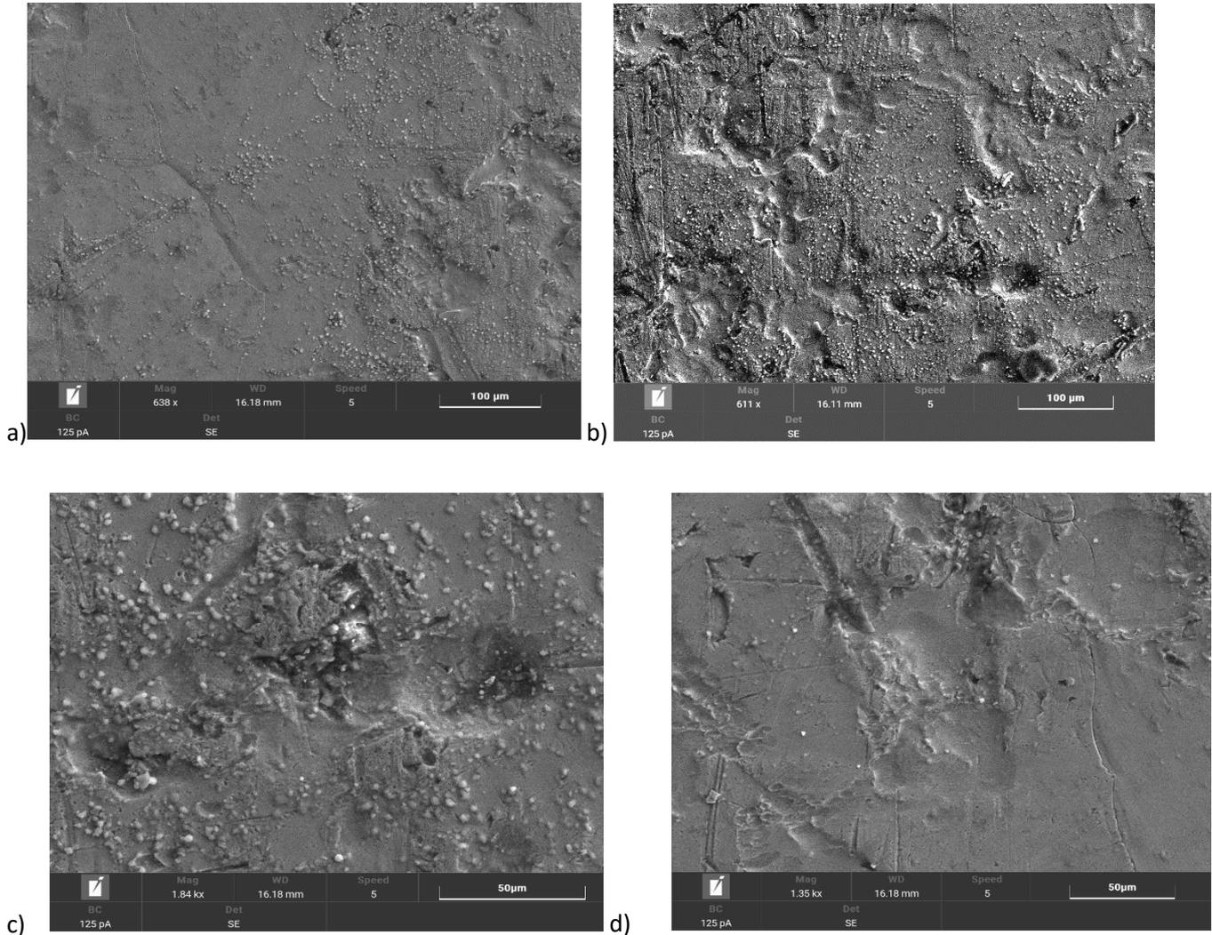
Figure. 5. Sheet surface without applied nano-insulation coating.
